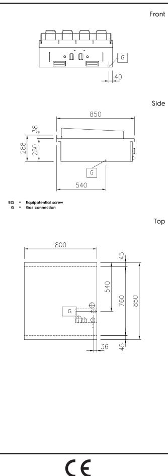
Gas Gas Power: 21 kW Gas Inlet: 1/2" **Key Information:** External dimensions, Width: 800 mm External dimensions, Depth: 850 mm External dimensions, Height: 250 mm Net weight: 110 kg One-Side Operated;Top **Configuration:** Grid dimensions: 728 mm
